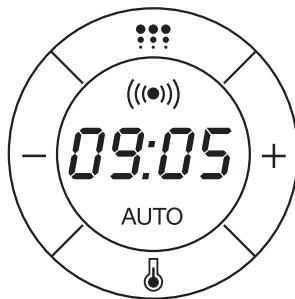
Symbol : Lights up when the Pyrolytic function is chosen
