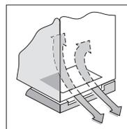
Pay attention to fix the ovens in an absolutely firm way, as above indicated, and to insulate the electrical elements in order to avoid an eventual contact with metallic parts.
