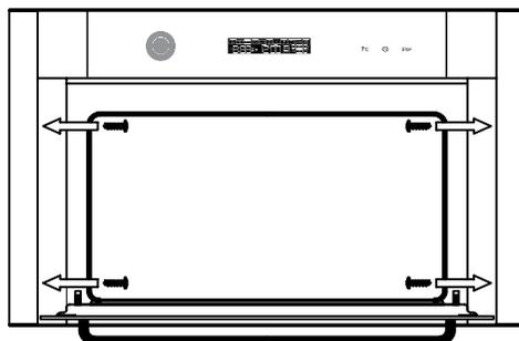
•The sides and the base surface where the oven is to be installed should be milled as shown in figure to allow a safe air intake and a free air circulation around the oven, thus granting its good operation and avoiding damages to the furniture.
