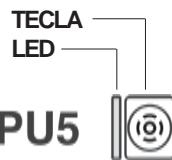
**PU5:** ON/OFF AUTOMÁTICO (Sensor)
