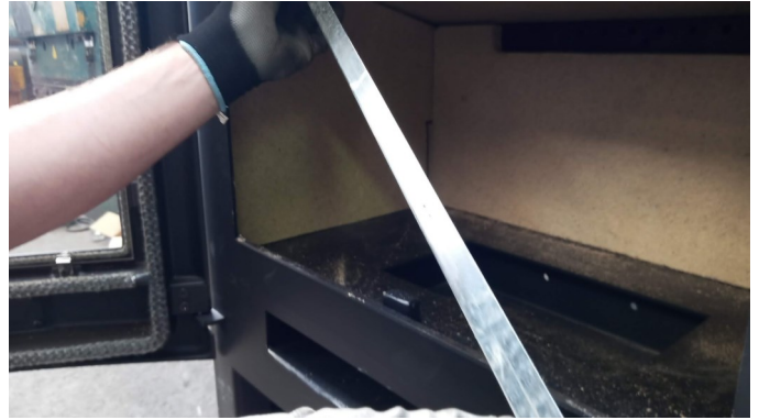
Keeping the top baffles raised, remove the left-hand side panel.
