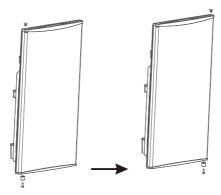
5)Install the door on the lower hinge assembly, and then install the upper hinge, hinge cover, pins and hole cap in sequence.
