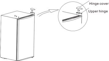
3)Remove the door first, then remove the lower hinge assembly and levelling foot, interchange the positions of the lower hinge assembly and levelling foot and install them.
