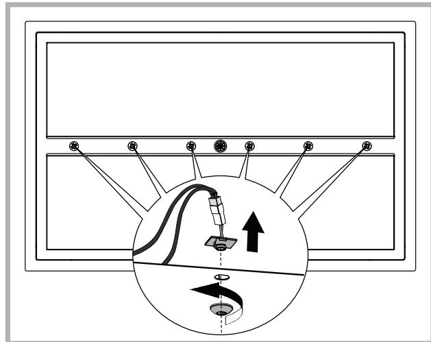
If the light spot is damaged, it must be replaced only by the manufacturer, its service agent or similarly qualified persons in order to avoid a hazard
