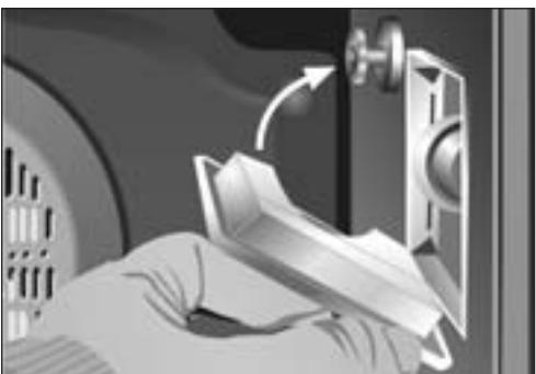
The replacement bulb must be resistant to temperatures up to 300 °C. You can order one from Technical Service.
