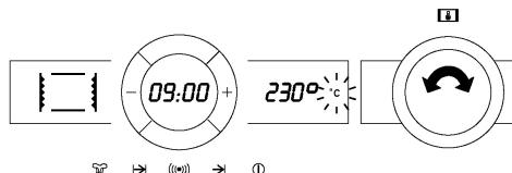
10. When the cooking cycle finishes, touch the sensor ①. The oven will turn itself off, just showing the current time.
