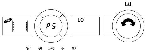
7. The following step is to confirm the weight of the food that is to be cooked. A weight will appear on the display for the recipe and the symbol "kg" will start flashing. Turn the temperature selector if you want to change the weight. Touch the sensor ② to confirm or else wait a few moments.
