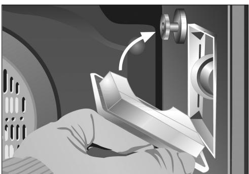
The replacement bulb must be resistant to temperatures up to 300 °C. You can order one from the Technical Assistance Service.
