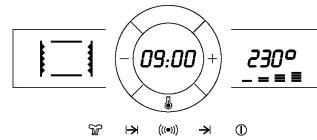
8. During cooking, symbol will light up to indicate that heat is being transmitted to the food. This symbol turns itself off when the selected temperature has been reached.
