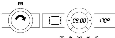
3. If you wish to cook at a different temperature, adjust the temperature selector. Failure to do so will mean that the oven will cook at the recommended temperature.
