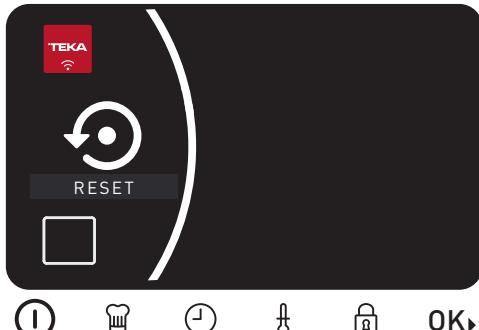
In this menu, press touch key **OK▶** to delete all the data and to restore the oven to the factory settings:
