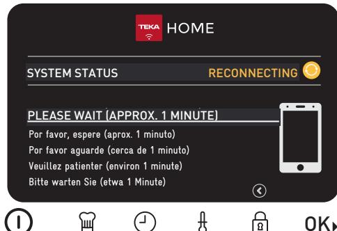
The oven will automatically try to reconnect to the previously configured Wi-Fi network. If the process is satisfactorily concluded, a connection correct message is displayed.
